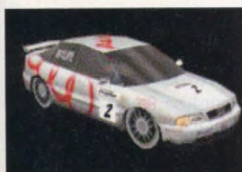
Audi A4 Drivers: Yvan Muller, John Bintcliffe Engine: 4-cylinder, 1998cc, 16V Output: 296bhp @ 8250rpm Drive: FF
