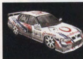
Nissan Primera Drivers: David Leslie, Anthony Reid Engine: 4-cylinder, 1998cc, 16V Output: 297bhp @ 8300rpm Drive: FF
