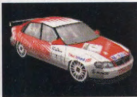
Vauxhall Vectra Drivers: John Cleland, Derek Warwick Engine: 4-cylinder, 2000cc, 16V Output: 295bhp @ 8400rpm Drive: FF
