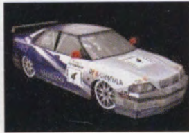
Volvo S40 Drivers: Rickard Rydell, Gianni Morbidelli Engine: 5-cylinder, 1999cc, 20V Output: 290bhp @ 8500rpm Drive: FF
