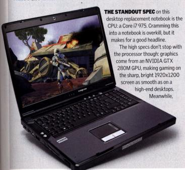
three hard drives optimise every loading time possible: a 80GB SSD blasts through booting, while two 500GB HDDs in a striped RAID array provide 1TB of data with fast access.
