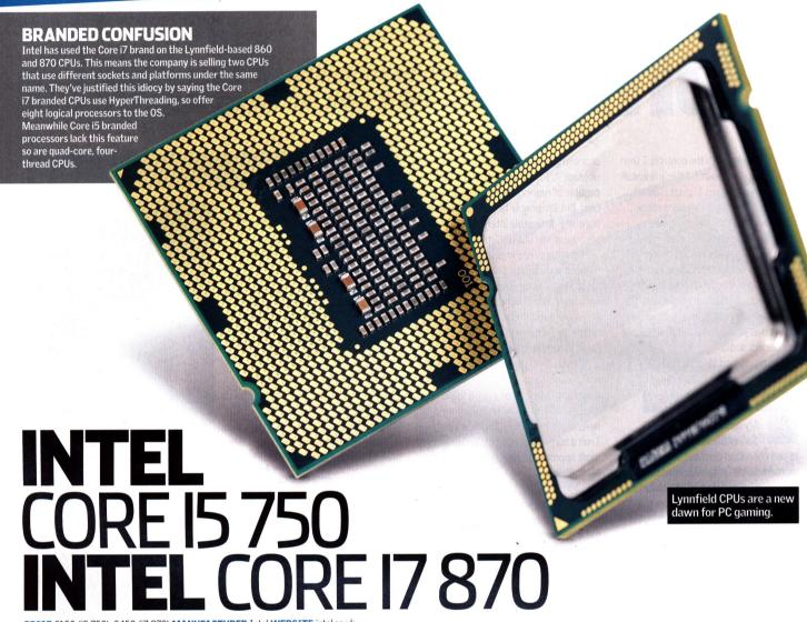
**NTEL'S NEW LYNNFIELD-class** CPUs - aka the Core i5 range make existing Bloomfield Core i7 processors seem rather redundant. These CPUs are based on the Nehalem design used in the Bloomfield Core i7 processors that were launched last year, but sport a few changes.
